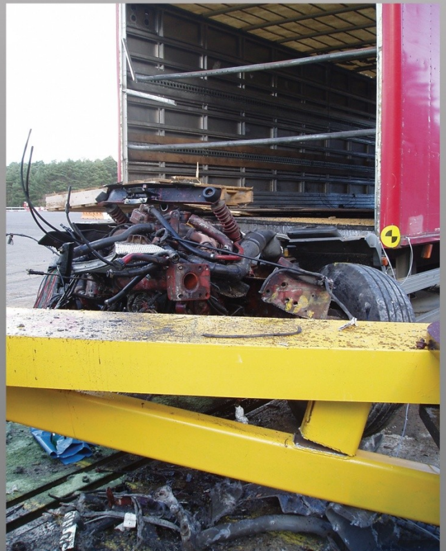
Terra Road Closer impact test results
